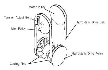
4. Retighten the tension adjust bolt 1/4 turn to set the lockwasher and prevent loosening of the tension adjust bolt.
